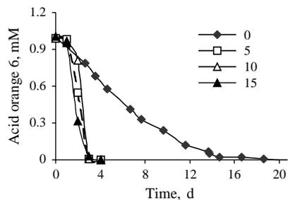
**Figure 4** Influence of riboflavin concentrations (numbers on graph in  $\mu\text{M}$ ) on acid orange 6 and anaerobic biodecolourisation (5 vol.% sludge)
