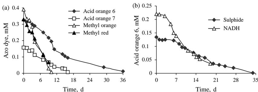
**Figure 3** Decolourisation of azo dyes by anaerobic culture broth devoid of cells (a) as well as sulphide and NADH (initial concentration of both – 0.5 mM) (b)
