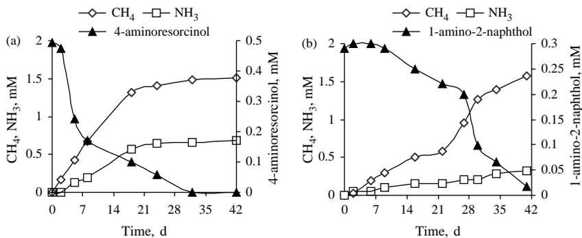
**Figure 6** Anaerobic biodegradation of 4-aminoresorcinol (a) and 1-amino-2-naphthol (b)
