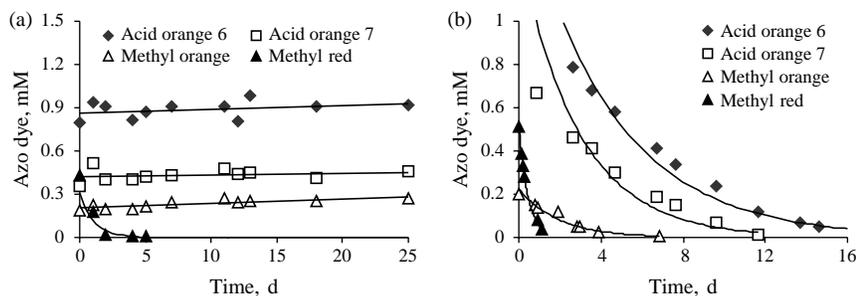
**Figure 2** Aerobic (a) and anaerobic (b) biodegradation of selected azo dyes
