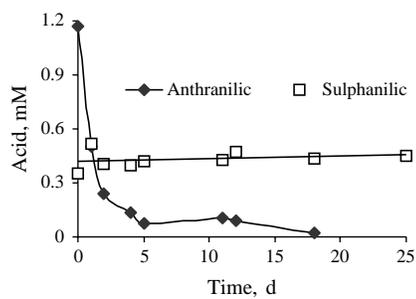
**Figure 5** Aerobic biodegradation of anthranilic and sulphanilic acids
